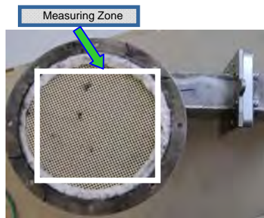
Fig. 10 Cylindrical multimode applicator with a Cordierite-DPF and soot load
