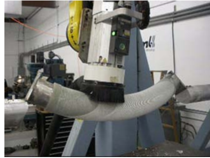
Figure 4. Bent DH dipole magnet being manufactured at AML
