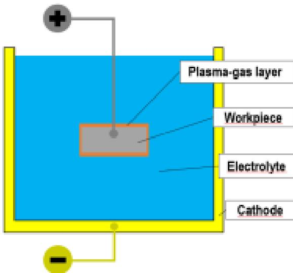
Figure 1: Principle scheme.
