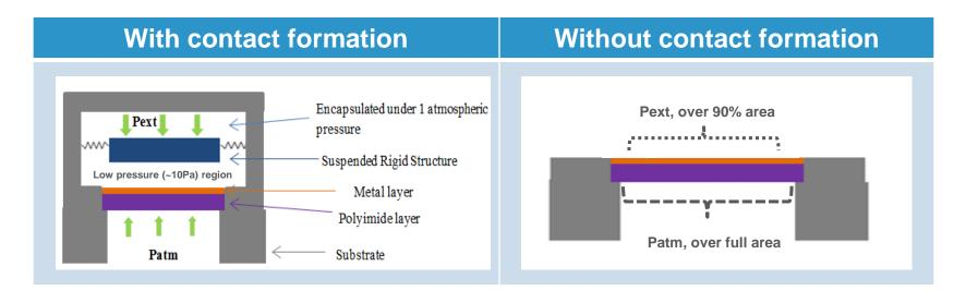
Patm, atmospheric load (acting over 100% area) and Pext, external load (acting over 90% area)
