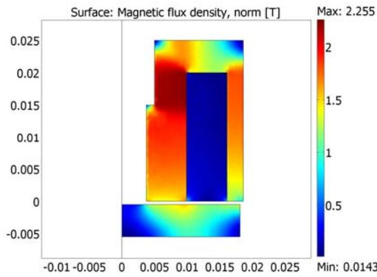
Figure 5. FEM Model of the EMVA.
