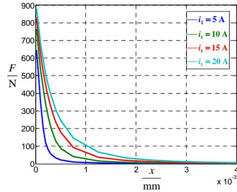
Figure 8. Electromagnetic force.
