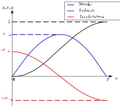
Figure 2. Used profiles for stroke, velocity and acceleration.
