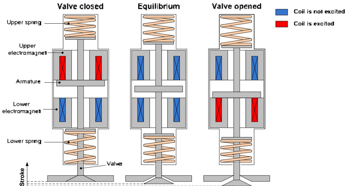
Figure 3. EMVA Principle of Operation.
