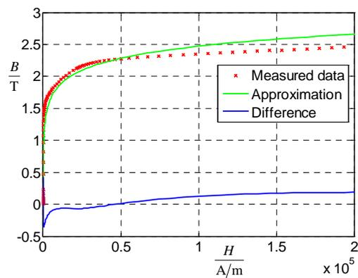
Figure 6. Used B-H curve.
