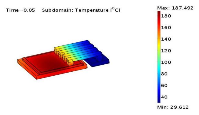
Metallization thickness of 30  $\mu m \rightarrow$  decrease of 52°C compared to the device with 4  $\mu m$
