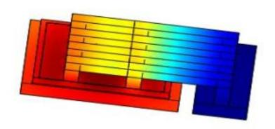
Temperature distribution after 50 ms  $T_{Max}$ = 169°C
