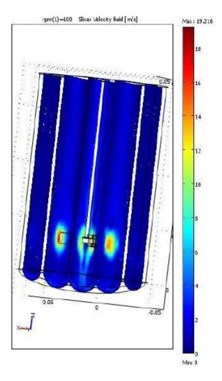
Figure 2: The simulation results of the stirred tank with a three bladed impeller.
