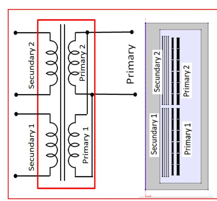
Two secondary windings are placed one above the other and feeding a rectifier (here not drawn). The primary, fed by the power line is accordingly split in two parts, so that each one is (mainly) coupled with the secondary winding in front of it.
