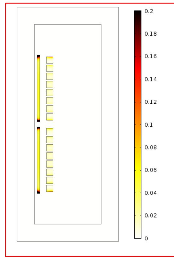
Figure 2 (left) shows the sum\*\* of the losses over the three frequencies. Color scale is saturated at 0.2[kW/dm^3] while peak value of this quantity arrives up to 3.4[kW/dm^3].
