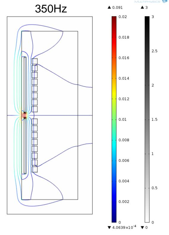
In Figure 1 a radial flux for the 5<sup>th</sup> and 7<sup>th</sup> harmonic is clearly visible looking at the streamlines. This is causing large and highly concentrated losses. Peak value for current density in each primary is 3.0, 1.1 and 0.9 [A/mm^2] respectively for 50, 250 and 350 Hz. While for the each secondary it is respectively 7.0, 11 and 10 [A/mm^2].
