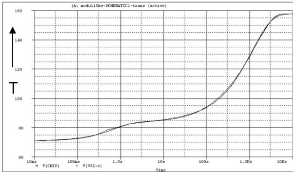
**Figure 2:** Zth-curves extracted and used in electrical network simulation.
