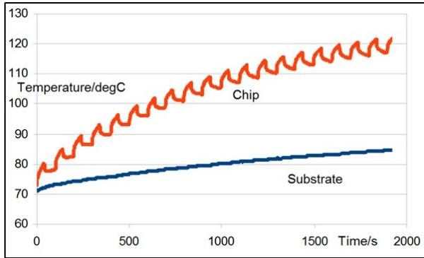
**Figure 3:** Dynamical behavior of converter in forklift driving scenario.
