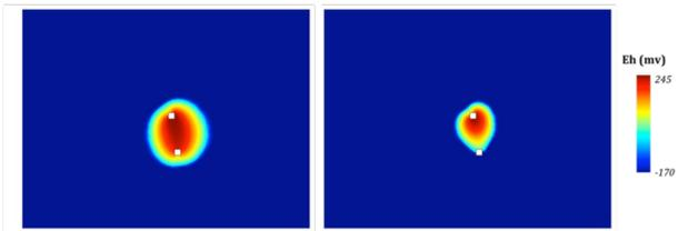
**Figure 3:** Redox plume after 2 days from the beginning of the experiment for a flow porosity of  $6 \times 10^{-4}$  (left) and  $1 \times 10^{-2}$  (right).
