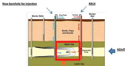
**Figure 1:** Set-up of the redox experiment. An oxygenated water is continually being injected (in the injection well) and extracted (in the pumping well).
