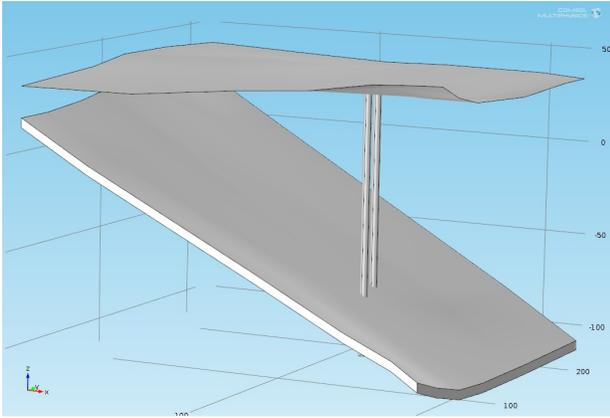
**Figure 2:** Representation of the soil surface, the transmissive zone HZInf7 and the two boreholes of the in-situ experiment.
