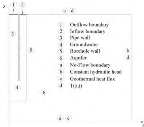
**Figure 2.** Simplified representation of a standing column well and boundary conditions of the model.
