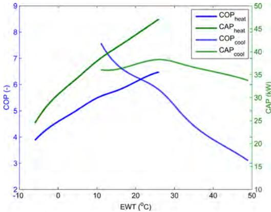
**Figure 3.** Interpolation functions used to describe the capacity ( $CAP$ ) and the coefficient of performance ( $COP$ ) of the heat pump used in the simulation.
