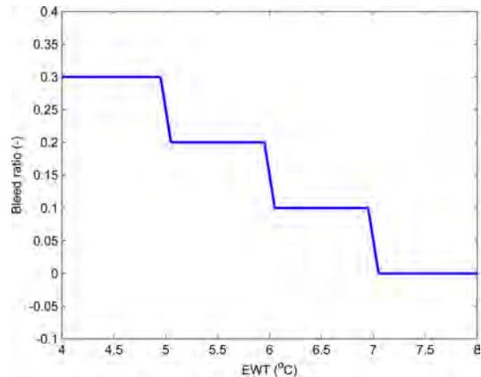
**Figure 4.** Function use to describe the bleed ratio as a function of  $EWT$ .
