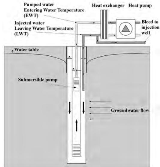
**Figure 1.** Illustration of a standing column well system
