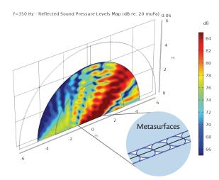
**FIGURE 5.** Reflected sound pressure levels with 32x32 unit cells at f = 350 Hz, for a prescribed reflected angle of 60°.
