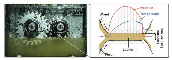
FIGURE 1. High-speed camera image of a dip-lubricated gear pair under operation (left) and schematic illustration of the EHL contact (right).
