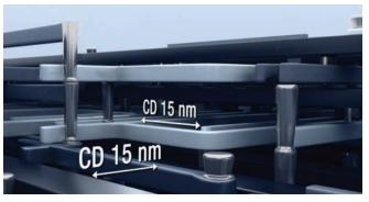
**FIGURE 1.** The critical dimensions inside a smartphone processor measures in nanometers. To put it in perspective, a human hair measures 5300 times larger than the critical dimensions in these chips.
