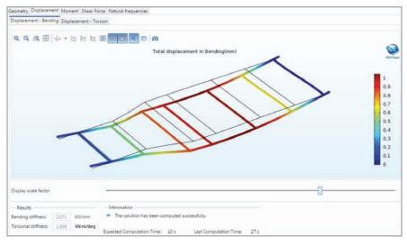
FIGURE 6. Simulation results obtained from the chassis app for a particular configuration.
