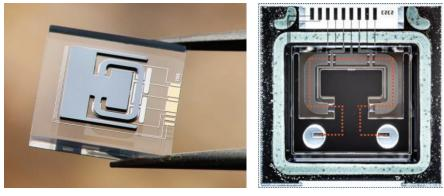
FIGURE 4. MEMS Coriolis chip used for density and viscosity measurements. Left: Complete sensor held by pliers. Right: Chip layout inside the device.
