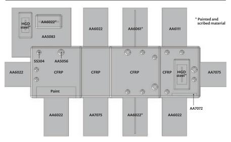
**FIGURE 5.** Multimaterial assembly built to demonstrate the relevance of using numerical simulation of corrosion to raise red flags for inappropriate designs.
