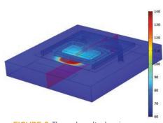
**FIGURE 6.** Thermal results showing temperature in the MEMS Coriolis chip.
