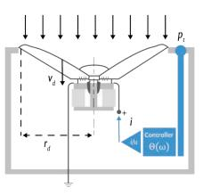
**FIGURE 3.** Illustration depicting the Active Electroacoustic Resonators (AER) concept.
