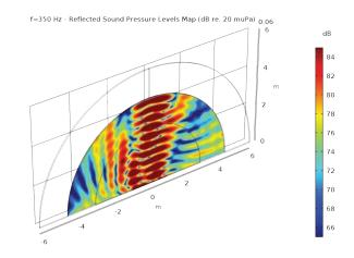
**FIGURE 6.** Reflected sound pressure levels with 32x32 unit cells, at f = 350 Hz, for a prescribed reflected angle of 0°.
