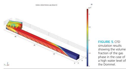
level on the flow profile. He was also able to determine the volume fraction of gas at any location throughout the channel, making it possible to understand the effectiveness of the aeration system (Figure 5).
