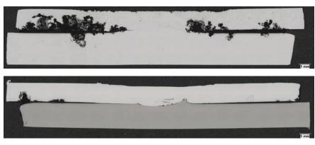
**FIGURE 3.** Cross-sectional view of multimaterial friction-stir welded (FSW) assemblies after a 100,000 km road exposure between a wheel and a mud flap. Top: Dominant crevice mechanism in a AA7000 series to AA6000 series FSW assembly, Bottom: Dominant galvanic corrosion in AA5000 series to stainless steel 300 series FSW assembly.
