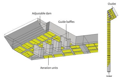
FIGURE 4. Geometry of the aeration channel. Aeration units are represented in yellow.
