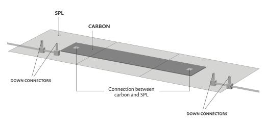
FIGURE 2. Geometry of the thin aluminum surface layer protection (SPL) placed on top of a carbon stack.
