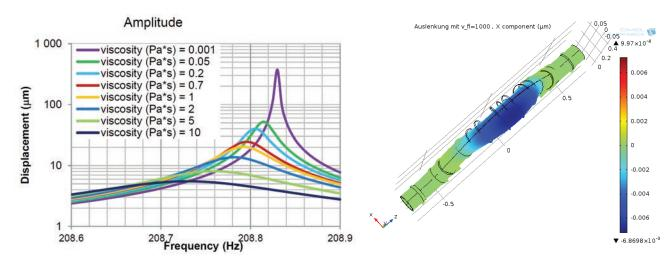
FIGURE 3. Simulation results showing the change in tube oscillating frequency for different fluid viscosities and the resulting mechanical displacement. At right is a visual example of tube deformation due to the oscillating motion.
