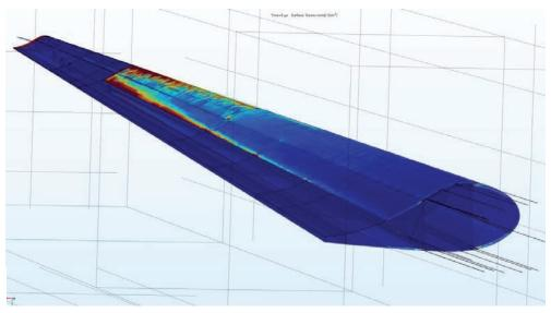
FIGURE 4. Simulation results showing the current density on a sample wind turbine blade made of several carbon stacks.
