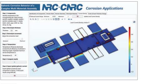
**FIGURE 9.** Simulation app for determining the galvanic corrosion behavior of a complex multimaterial assembly. Top: Visualization of the electrolyte potential across the assembly. Bottom: Visualization of current density throughout the assembly.
