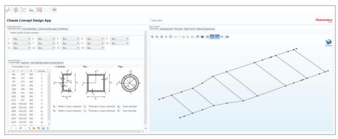
FIGURE 5. The user interface of the chassis simulation app available on Mahindra's internal portal, called MathApps.
