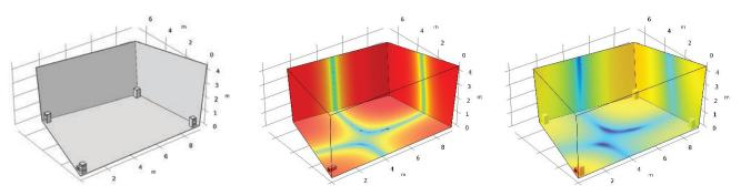
FIGURE 2. Left: Geometry of the reverberant chamber with four AER prototypes at the 4 corners. Middle and right: Sound pressure level distribution in the chamber excited on mode 110 at 35.3 Hz without and with absorbers, respectively.
