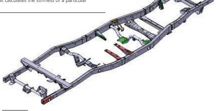
FIGURE 4. Geometry created in CATIA® software representing the structure of a typical utility vehicle chassis.
