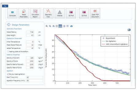
FIGURE 2. Simulation app that calculates drying times for models with no agitation (green) and intermittent agitation (red) and compares them with an experimental result.
