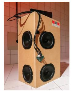
**FIGURE 1**. Active Electroacoustic Resonator prototype. Image credit: EPFL/Alain Herzog.
