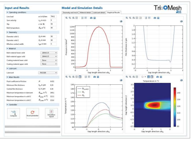
FIGURE 2. This custom simulation app packages a complex, coupled physics solution to TEHL into an easily accessible tool for everybody in the research center to use.
