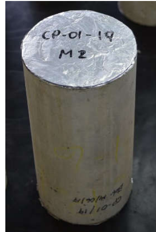
Figure 1. A cylindrical sample of concrete with its bases covered by aluminium foils.
