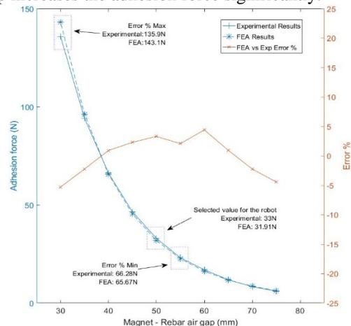
Figure 8. Comparison between experimental results and FEA from COMSOL.
