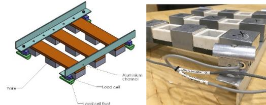
**Figure 11.** Test rig construction with 4 load cells.
