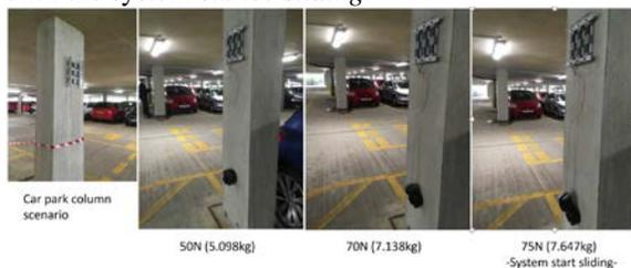
**Figure 12.** Test in a real reinforce concrete structure: car park column.
