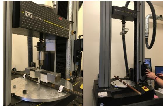
Figure 7. In house test rig using an Instron machine (2kN tension/compression load cell).
