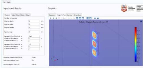
**Figure 4.** Three N52 magnets arranged N-S-N.
