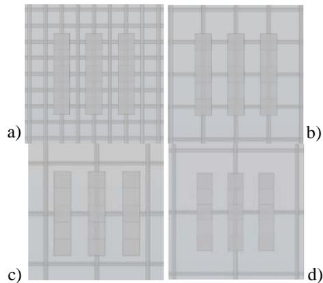
**Figure 10.** Rebar mesh spacing in 4 configurations: a)50x50mm, b)100x100mm, c)150x150mm, d)200x200mm
