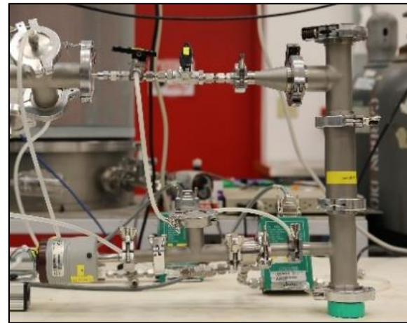
Figure 2: Fluidized dust bed to inject dust particles into the ESP
