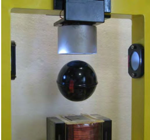
Figure 4. MLS2EM [3] - upper electromagnet replaced with cylindrical one.
