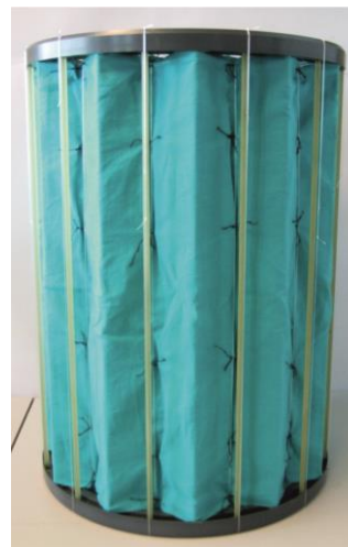
(b) Spacer with fabric to cover thermal cylinder
