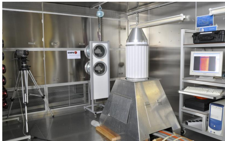
(a) Thermal cylinder inside the climatic chamber
