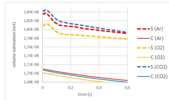
**Figure 6** volume variation estimation after laser cut-off for various gas
