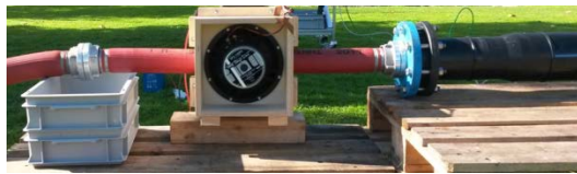
Figure 2. Part of the test bench to measure phase velocities in water pipes. A public hydrant fills the pipe with water by means of a fire hose (on the left). A loudspeaker box encloses the 8 bar-pressurized hose and generates the white noise signal (center). The signal propagates along the pipe on the right.
