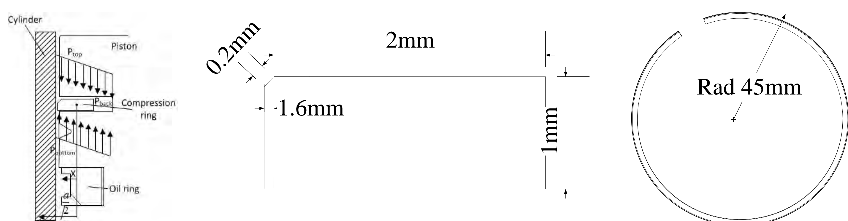
Figure 2a Showing mathematical model (left). b Showing ISO 6622-1 Internal combustion engines cast iron standard (centre). c showing ring OD (right).
