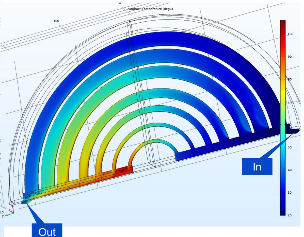
Temperature distribution of an eroded Silicon target bonded with Indium
