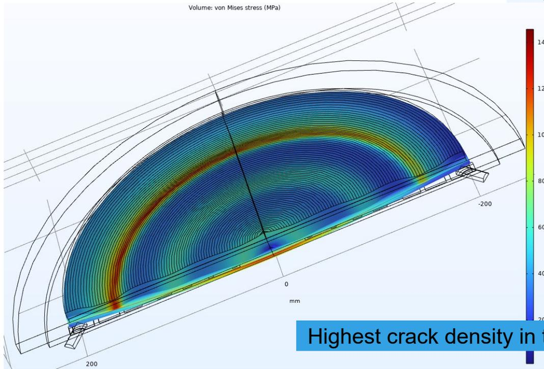
Highest crack density in the erosion groove
