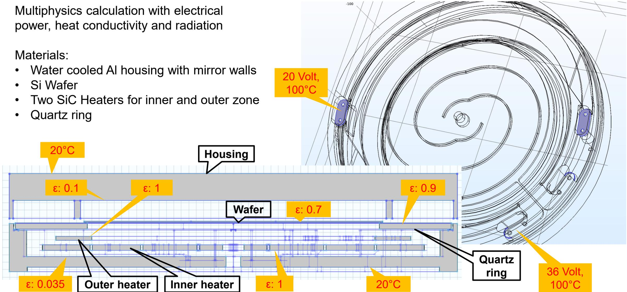
Temperature of the 2 SiC-heater circuits
