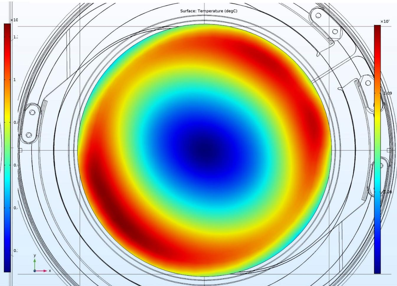
In sputtering very high heat loads of up to 320'000 W/m<sup>2</sup> on the target must be cooled efficiently by a cooling structure as flat as possible, since magnets have to be applied at the back side of the cooling plate as close as possible. Also, the cooling plate must withstand water and atmospheric pressure.
