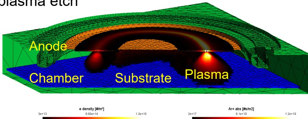
Monte Carlo software for simulation on substrate features incl. collisions, sticking coefficients and surface diffusion
