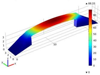
Surface: Total displacement (nm) Surface Deformation: Displacement field
