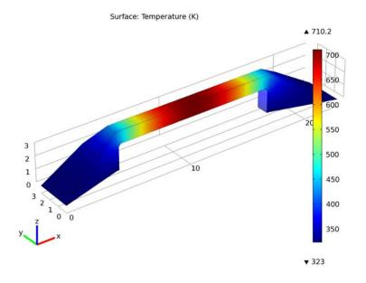
Figure 2: Surface temperature with temperature-dependent electric conductivity. Surface: Total displacement (nm) Surface Deformation: Displacement field
