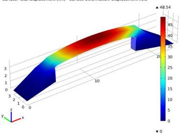
Figure 3: Microbeam deformation with temperature-dependent electric conductivity.
