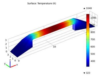
Temperature field for constant electric conductivity.
